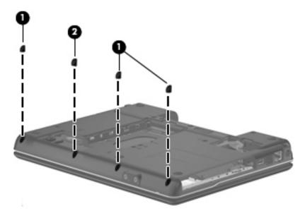
3. Remove ten Torx T8M2.0×6.0 slotted screws.
